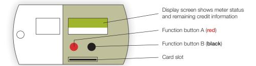
This meter is operated by a Quantum Card. To function properly this card must be registered with the meter. Cards can only be obtained from your gas supplier.
